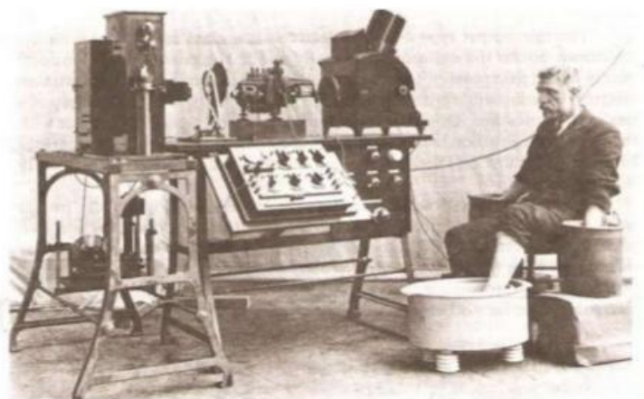
Figure 1 ECG measurement using immersion electrodes. Original Cambridge electrocardiograph (1912) built for Sir Thomas Lewis.
